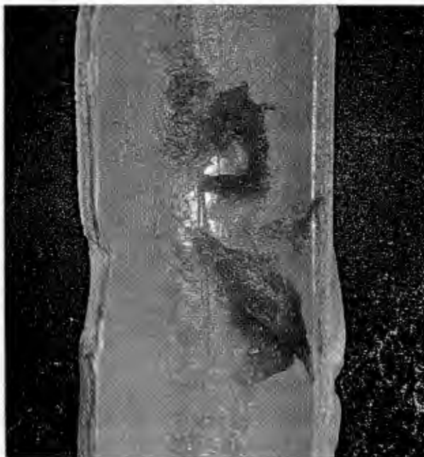
Figure 11 – Material observed at inner surface of failed CPVC pipe exposed to a mixture of water and bio-glycerin.
