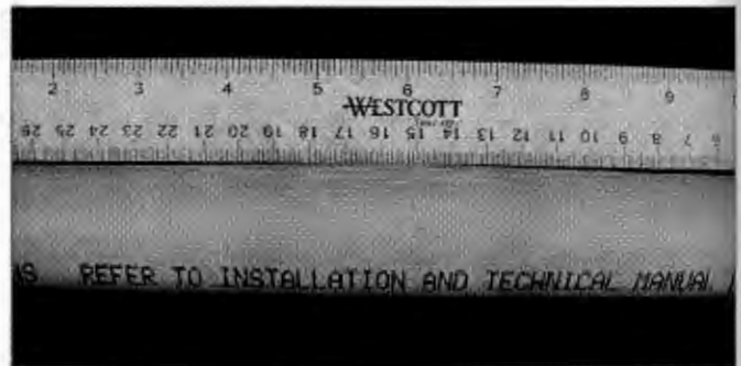
Figure 4 – Bulging of a failed CPVC pipe exposed to a mixture of water and bio-glycerin.
